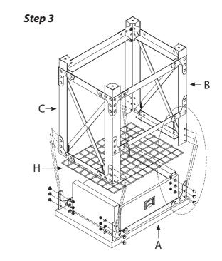
**Note:** Assemble upside down according to instructions. Ensure workbench top is flat on the floor.
